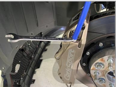
For proper brake bleeding, always start with the bleed screw furthest from the master cylinder. In this case we start with the outer bleed screw on the passenger side, then passenger inner, driver outer, and finally driver inner.
