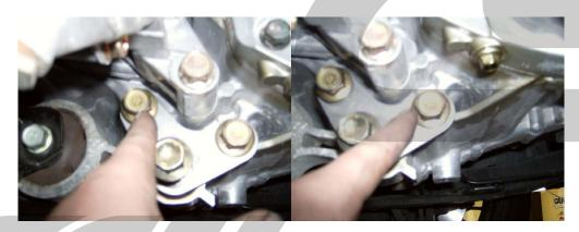
Step 36: Tighten the 17mm headed bolt on the lower engine torque mount to 55-76 ft-lbs
