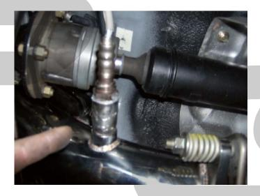
Step 42: Put a small amount of anti seize on the upper O2 sensor threads and re-install the upper O2 sensor. Route the wires along the same path as when they were originally at the firewall.
