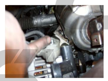
Step 24: Disconnect the alternator plug.
