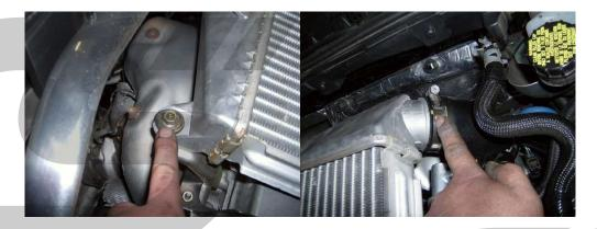
Step 4: Remove the vacuum hose to the bypass valve using the pliers to pinch the clamp open on the tabs. Remove the hose clamp on the large hose which connects to the bypass valve. Some effort may be required to remove the hoses once the clamps are removed.
