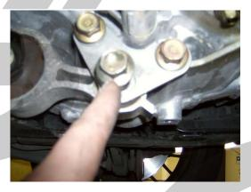
Step 35: Tighten the two 19mm headed bolts on the lower torque mount bracket to 49-68 ft-lbs.
