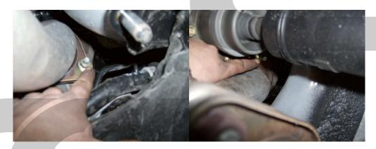
Step 17: For easy of removal take the two studs out of the catalytic converter and remove the mid pipe.
