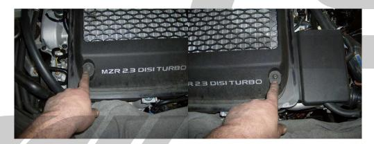
Step 3: Remove the three 12mm nuts that hold down the intercooler. Two of them are located on the front of the intercooler and one is located at the back. Disconnect the two intercooler hoses located on either end of the intercooler with the 10mm socket to remove the clamps. The rear clamp is also shown in the pictures below.
