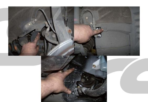
Step 21: Note how the belt is routed on the engine before removal to aid in re-installation. Take the 14mm wrench and turn the belt tensioner clockwise to release tension on the belt. Remove the belt.
