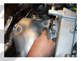
Step 56: Mount the 2 wiring clips to the bracket.
