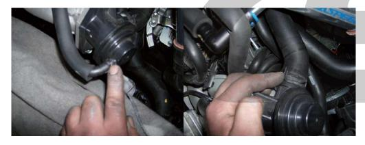
Step 5: Once the hoses are all loose carefully lift out the intercooler. Be careful not to damage the fins on the intercooler and set it aside in a safe place.
