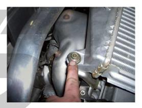
Step 59: Re-install the intercooler cover and re-install the two 10mm bolts.
