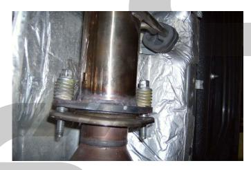
Step 44: Re-install the lower cross bar with the four 17mm headed nuts and tighten them to 55-79 ft-lbs. (Install option) Install two (2) of the supplied washers to each of the 4 studs on the cross bar if you need a little bit of extra clearance between the bar and the downpipe.
