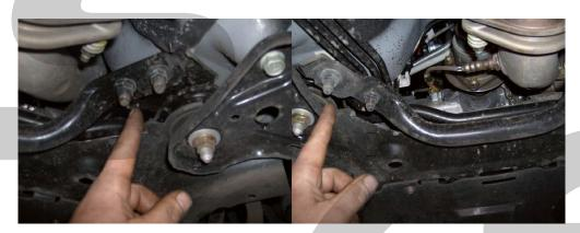
Step 15: Remove the two 14mm headed nuts and springs from the exhaust system to the mid pipe.
