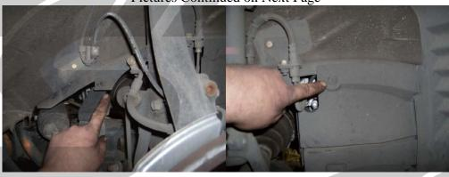
Step 51: Re-install the passenger side wheel liner and under tray.
