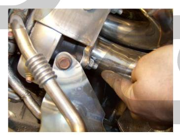
Step 40: Install the remaining four 14mm headed nuts and tighten in a criss cross pattern to 39-46 ft/lbs.
