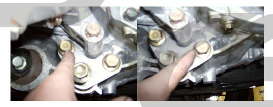
Step 30: Remove the 17mm headed bolt and let the mount swing down.
