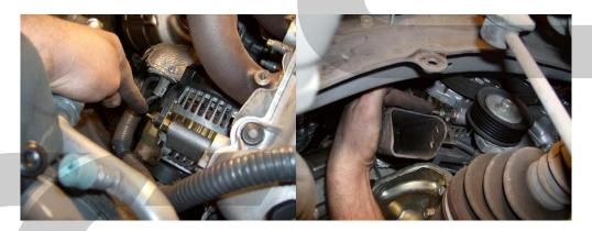
Step 49: Re-install the accessory drive belt on its original path.
