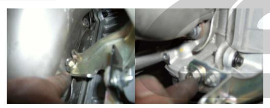
Step 55: Re-install the upper exhaust manifold heat shield with the original five 8mm headed bolts.
