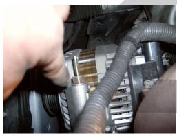
Step 46: Re-connect the electrical plug into the alternator.
