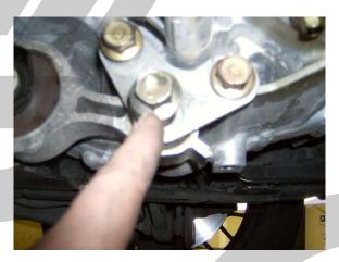
Step 31: Place the floor jack under the passenger side of the oil pan and remove the 17mm headed bolt from the top engine mount.
