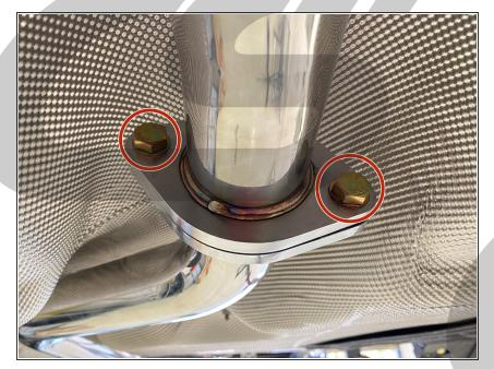
Align the midpipe flanges so they are even and tighten the bolts that connect the front and rear midpipe sections to 45 ft-lb using a 17mm socket and wrench.
