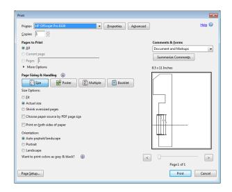
Print a copy of the drawing, making sure that the "Size Options" is set at "Actual Size" (or make sure "Scale" is at "100%")
