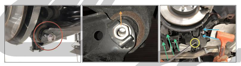
A Do not perform the next step until you are confident the 17mm lower control arm bolt is secure.
